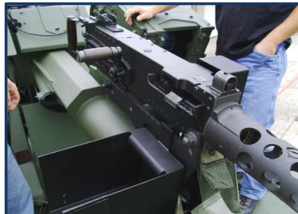
Step 4 – INSTALL SUB-CALIBER WEAPON INTO MOUNT ASSEMBLY.
