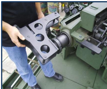
Step 3 – INSTALL GTS-30 MOUNT ASSEMBLY INTO Mk44 CANNON.
