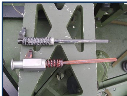
Step 2 – REPLACE THE Mk44 FIRING PIN WITH A DUMMY FIRING PIN.
