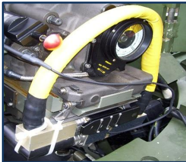
Step 1 – INSTALL THE HOM AND FCIB TO THE Mk44 CANNON.
